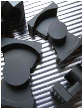
Core for built-in DC-DC converter's main transformer for HEV, EV, and FCEV Example of core shape (one pair) L35×W26×T35mm / L41×W28×T30mm
